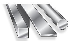
Ameralloy W1 is a straight carbon water hardening tool steel available in a wide range of carbon content. It is a shallow hardening steel – a case hardness of Rockwell C 66 can be attained for excellent abrasion resistance and a softer core for superior toughness.
