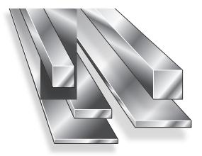
Durelloy Key Stock bars are sharp-cornered with parallel sides, for applications such as keys, tool shanks gauges and wear strips. For areas requiring close tolerance and high tensile strength. All bars are cold drawn.
